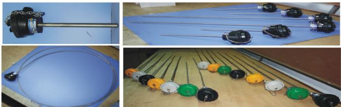
M.I. Thermocouple With IP-65 / IP-67 Die Cast Aluminum Head Are Available From Outer Diameter of 3.0mm, 6.0mm, 8.0mm. For Connection to The Extension Cable There is a Ceramic Terminal Block Inside The Head. Length of sensor should as per customer requirements. Sheath Materials are selected depending upon operating temperature & application of uses. Instrument connection should provide as per customer need. The Sensor Can Be Custom Manufactured to Suit Your Exact Application Requirements.
