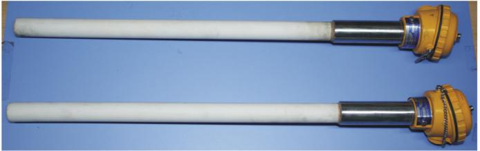
Ceramic Sheath Thermocouple With IP-65/ IP-67 Die Cast Aluminum Head Are Available From Outer Diameter of 12mm, 20mm, 32mm & also as per customer Requirements. For Connection to The Extension Cable There is a Ceramic Terminal Block Inside The Head. Here Ceramic Sheath is Inserted into a Metal Support Tube & Thermocouple Element Insulated By Ceramic Sleeves. Flange should provide as per customer need. The Sensor Can Be Custom Manufactured to Suit Your Exact Application Requirements.
